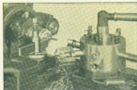
Fig. 13. Draw-in Collet Chuck and Turret for Making Small Parts.
