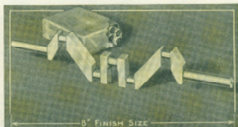
Fig. 24. Crankshaft of a Small Marine Motor, Cut from a Solid Bar and Machined on a 9-inch Junior Lathe. Actual Size of Crankshaft is 8 Inches Long.
