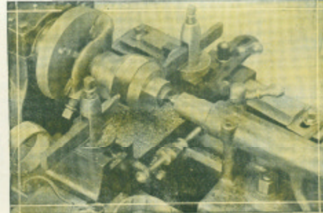
Fig. 71. Lathe Equipped with Double Tool Slide, Turning Two Diameters at Once.
