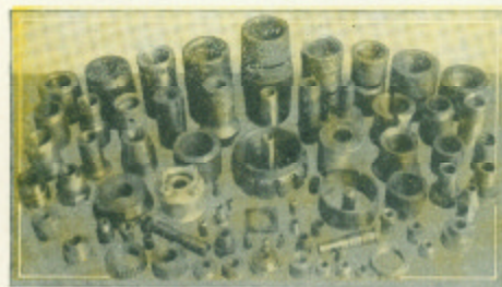
Fig. 32. Bushings of All Kinds Can Be Made on the 9-inch Junior Lathe.
