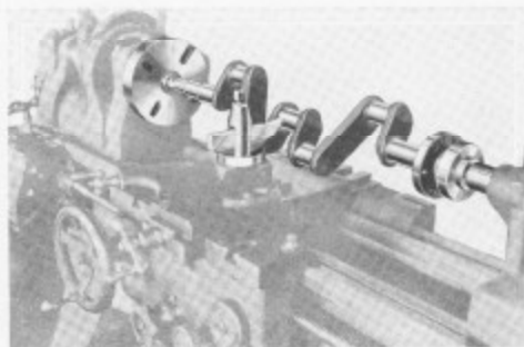
Fig. 111. Truing the Main Bearings of a Crankshaft
