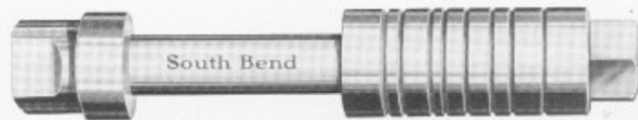
Fig. 60. Self-Centering Straight Mandrel with Spacing Collars and Nut
