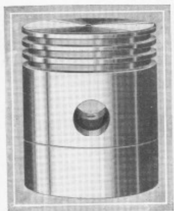
Fig. 42. Close-Up of Piston after Being Finish Turned in the Lathe
