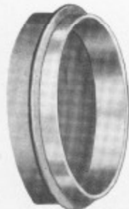
Fig. 87. Metal Liner Partly Fitted in a Brake Drum
