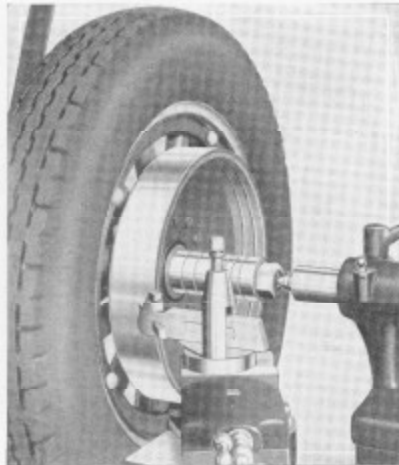
Fig. 71. Truing an External Band Brake Drum Mounted on a Straight Mandrel with Universal Bearing Adapters
