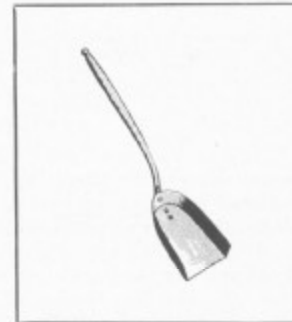
Figure 40—Small Fire Shovel. In making this project experience is gained in upsetting, bending, drawing, punching and riveting. Price: 1 Blue Print, 1 Job Sheet, 25c.
