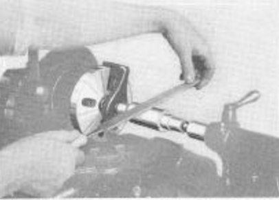
Fig. 42. Lathe is Practical for Filing, and Polishing Bushings, Shafts, Parts, etc.
