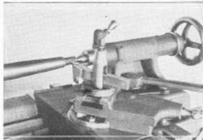
Fig. 32. Cutting a Screw Thread on an Axle. Screw Thread Range of Lathe, 4 to 40 per inch.
