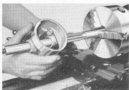
Fig. 41. Using Lathe as a Variable Speed Reamer Driver Ream Wrist Pin Hole.
