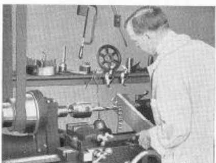
Fig. 35. Lathe used as Drill Press for Drilling Hole in Flat Piece of Work
