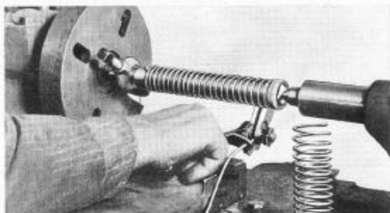
Fig. 17. Winding a Valve Spring.
