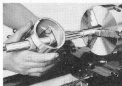
Fig. 25. Using Lathe as a Variable Speed Reamer Driver, Reaming Wrist Pin Hole.
