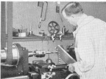
Fig. 26. Lathe used as Drill Press for Drilling Hole in Flat Piece of Work.
