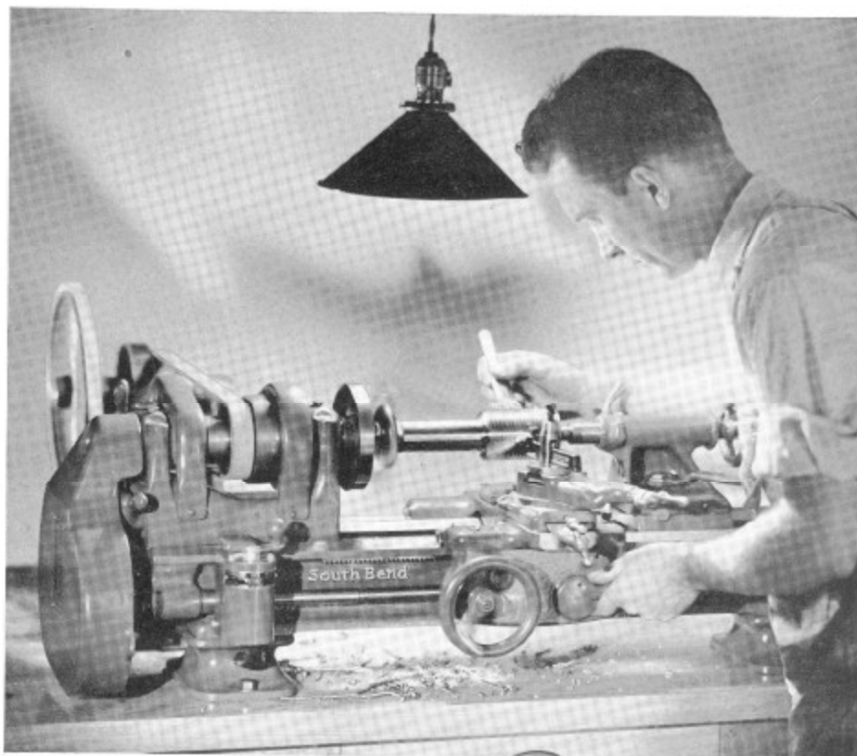
Fig. 29. Applying lard oil to work with small paint brush while cutting screw threads in a tool steel thread gage.
