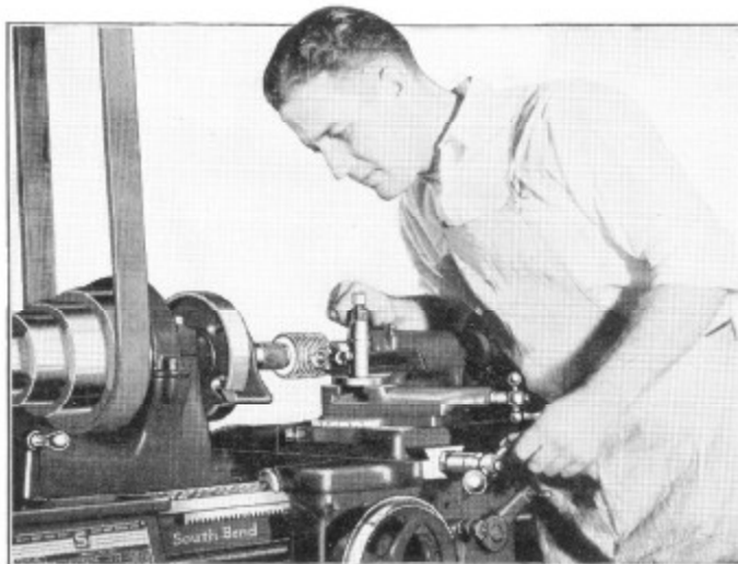
Fig. 1. Cutting a Screw Thread in the Lathe.
