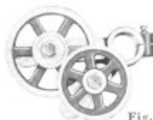
Fig. 42. Metric Transposing Gear Attachment for 16" Lathe.
