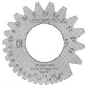
Fig. 14. Standard screw thread tool gage for grinding threading tools.
