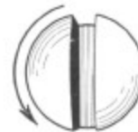
Fig. 37. A left hand screw advances when turned counter-clockwise.
