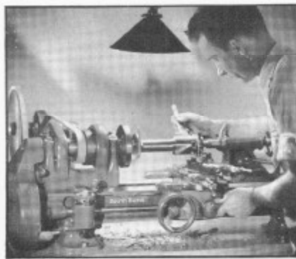
Fig. 15.—Cutting Screw Threads
