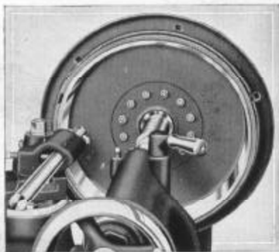
Fig. 18. A Lincoln car brake drum being trued by turning in the lathe.
