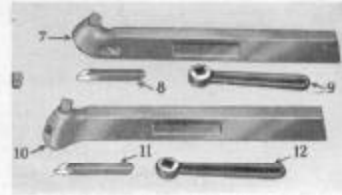
Fig. 23. Right and left hand tool holders with extra long shanks for truing brake drums.
