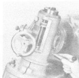
Fig. 9. Turn worm to move head to vertical position.
